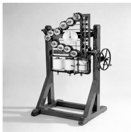
The Kelvin tidal computer is an example of what we now would call an 'analogue computer'. Once set up with data from previous tidal events, it could calculate with great accuracy the height of future tides. It was so good that it was used for the tidal calculations for the D-day landings, and similar computers were used until the 1960's. At this point they were replaced by the modern electronic computer which we will discuss next.
